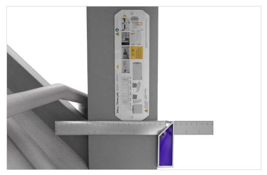
**Technique 2:** Visually, place the template in the desired installation location. Using a level, check that the template is level.
