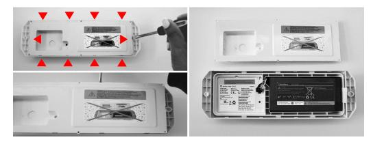
3. Disconnect the battery cable from the battery connector.
