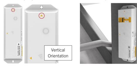
6. Insert your fastener of choice into the holes and use the appropriate tools to secure the module to the asset.
