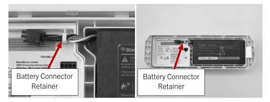
5. Place the battery cover onto the module. Place the screws in the circular recess on the battery door and cover with tape. Leaving the screws uninstalled is recommended as an indicator to the recipient that the battery is disconnected and must be connected before its next use. Module is now ready for placement into the UN certified Dangerous Goods packaging.
