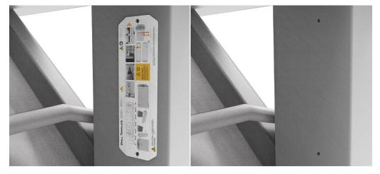
5. Ensure the arrow on the top of the housing is pointing to the sky. Place the module on the door, aligning the holes on the module with the holes you drilled into the door.
