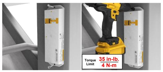
Do not over-tighten the fastener. Do not tighten fastener beyond 35 in-lb. (4N-m).
