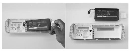
5. Place the battery cover onto the module. Place the screws in the circular recess on the battery door and cover with tape. Leaving the screws uninstalled is recommended as an indicator to the recipient that there is no battery installed and must be installed before its next use. Module is now ready for placement into the UN certified Dangerous Goods packaging.
