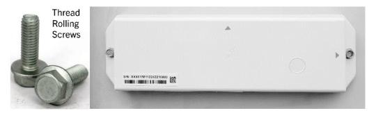
Thread rolling screws create their own threads within the thickness of the asset's installation surface. These threads allow the module to be secured to the asset, without the use of a secondary fastener, like a lock nut (although some thread rolling screws can be used with some lock nuts, for extra holding opportunity).
