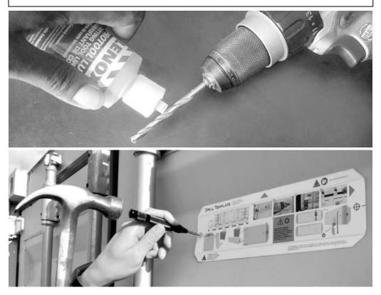
4. Remove the template. You now have two holes in the post. If there are any burrs around the holes, remove them at this time. Also, remove any dust or debris left over from the drilling or de-burring operations and ensure surface is clean and dry.
