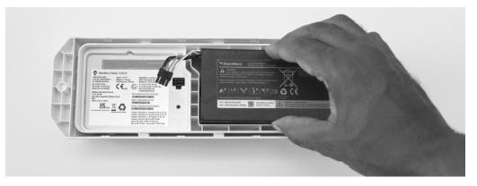
2. Connect the battery cable to the battery connector. The LED will blink to indicate the module is active. NOTE: It can take between 20-30 seconds for the blink sequence to begin. Please be patient. Once you see the LED blink, continue to the next step.
