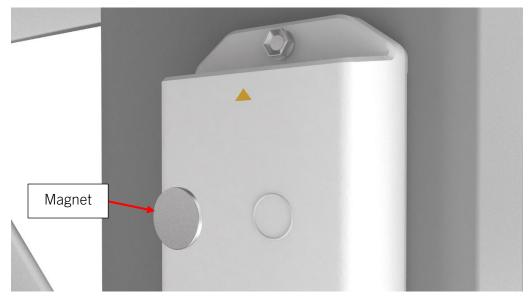
2. Place the magnet within the magnet ring on the front of the housing. Hold the magnet within the magnet ring for at least 5 seconds, then remove the magnet from the module. The module will reboot and reconnect to the cellular network within 5 minutes.
