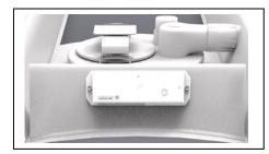
SPECIAL NOTE: To preserve the Intrinsic Safety of the BlackBerry Radar H2M IS module, if the module is dropped at any point during the handling or installation process, please replace with a different module that has not been dropped.
