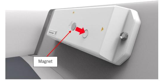
2. Place the magnet within the magnet ring on the front of the housing. Hold the magnet within the magnet ring for at least 5 seconds, then remove the magnet from the module. The module will reboot and reconnect to the cellular network within 5 minutes.
