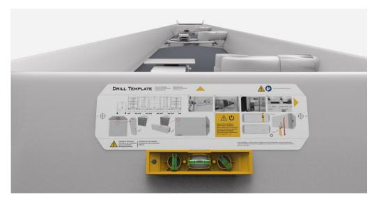
3. Using a drill bit, drill a hole through each of the cross hairs on the template. This will create two holes you will use to mount the module.
