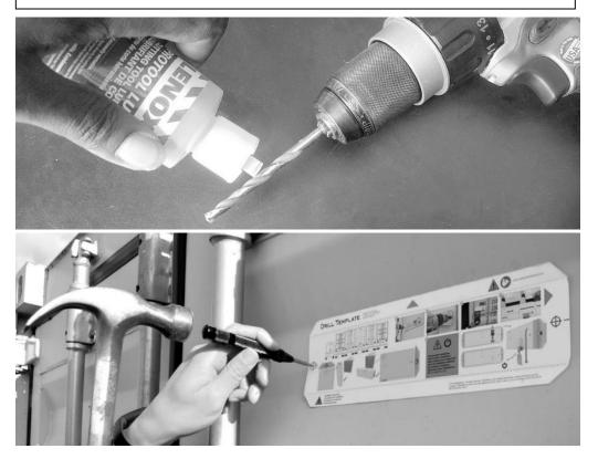
4. Remove the template. You now have two holes in the asset. If there are any burrs around the holes, remove them at this time. Also, remove any dust or debris left over from the drilling or de-burring operations and ensure surface is clean and dry.
