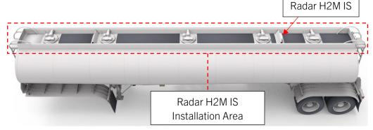
• The module may be placed on either side of the vertical walls along the top edge of the tanker. If placing along the interior surfaces of the vertical walls, near the manway lid, please consider how the manway opens. Do not install the BlackBerry Radar H2M IS module in an area where the manway lid operation or entry/exit to the manway is impeded.
