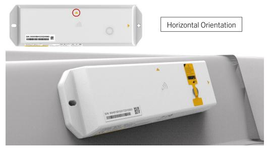
Insert your fastener of choice into the holes and use the appropriate tools to secure the module to the asset. Do not over-tighten the fastener/ tighten fastener beyond 35 in-lb. (4N-m).
