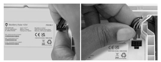
4. Store the battery cable by placing the battery cable under the battery connector retainer. **NOTE:** Battery cable must be stowed for transit to prevent unintended contact with the battery terminals.
