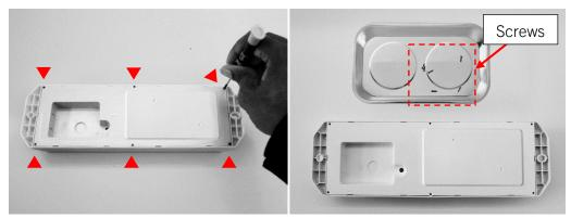
**Tip:** The use of a Magnetic Parts Tray is recommended to collect the screws.
