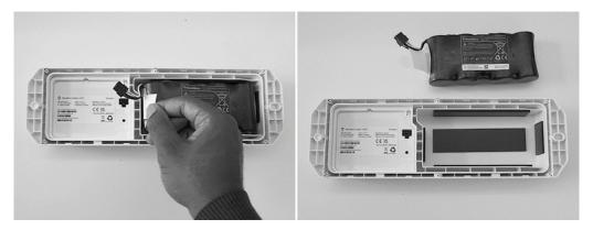
5. Without the battery installed, place the battery cover onto the module. Place the screws in the circular recess on the battery door and cover with tape. Leaving the screws uninstalled is recommended as an indicator to the recipient that there is no battery installed and must be installed before its next use. If no battery is installed, devices may be shipped in non-Dangerous Goods packaging.
