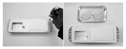
2. To separate the battery door from the outer housing—begin by inserting a flat screwdriver (3-7mm width) into the far-left or far-right slot, marked with the arrows, and pry upwards. Complete the battery door removal by working your way around the door-inserting the screwdriver into the other slots and prying upwards, until the door is free.
