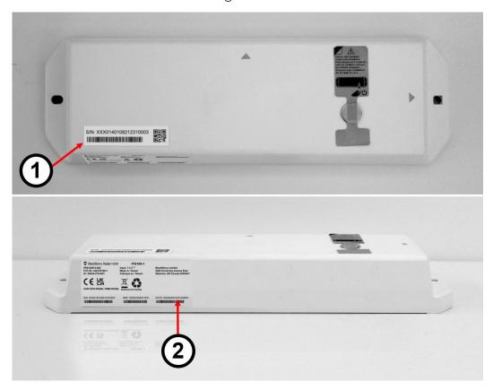
2. Once you have installed the module on the asset, create a record of the module-toasset-to-accessory pairing within the BlackBerry Radar Mobile App by recording the asset identifier and scanning the module identifier for the BlackBerry Radar H2M device and associated accessories.
