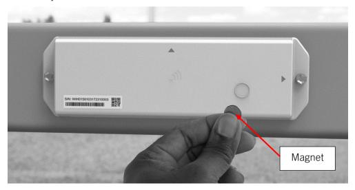
2. Place the magnet within the magnet ring on the front of the housing. Hold the magnet within the magnet ring for at least 5 seconds, then remove the magnet from the module. The module will reboot and reconnect to the cellular network within 5 minutes.
