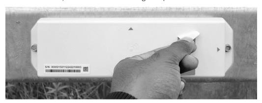
B. Continue to lift the magnet tape and fully remove the magnet tape from the module. Lifting the magnet tape will remove the magnet from the magnet ring.
