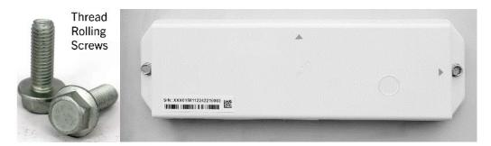
Thread rolling screws create their own threads within the thickness of the asset's installation surface. These threads allow the device to be secured to the asset, without the use of a secondary fastener, like a lock nut (although some thread rolling screws can be used with some lock nuts, for extra holding opportunity).
