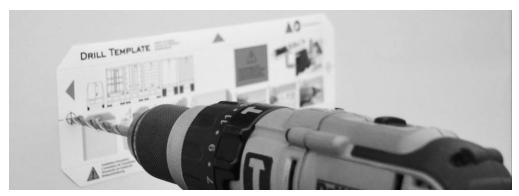
3. After drilling the holes and removing your template, install the well nut into the holes.
