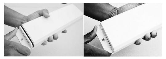
5. Locate the Fastener Bag and remove the two screws. Using a Phillips screwdriver, install the screws to secure the inner housing to the outer housing. **IMPORTANT:** Screw torque must be 3-3.5 in-lb. (0.35-0.4 N-m).
