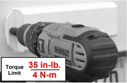
Do not over-tighten the fastener. Over-tightening can over-compress the mounting pad, which can damage the pad. Do not tighten fastener beyond 35 in-lb. (4N-m).
