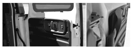
**Tip:** On some vehicles, where the planned mounting location is in front of a latch, you may want to verify the suitability of the area for mounting by checking behind the interior door panel.
