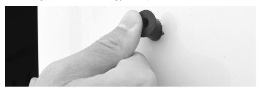
4. Place the module on the door, aligning the holes on the module with the holes in the well nut. Insert your fastener of choice into the holes on the module and well nuts. Use the appropriate tools to secure the module to the asset.
