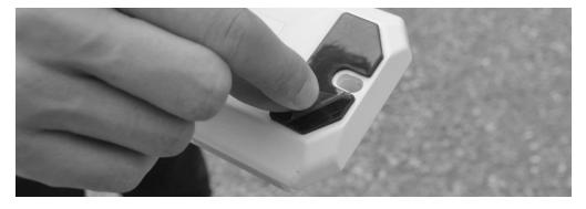
6. Place the module on the door, aligning the holes on the module with the holes you drilled into the door. To engage the adhesive, press the module firmly against the installation surface for 30-45 seconds.
