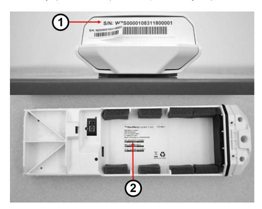
2. Once you are ready to install the module to the asset, remove the partially attached label from the front surface of the inner housing and place it on your worksheet, next to the asset identifier the module will be paired with.
