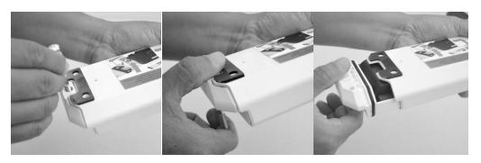
3. Remove the battery connector from the connector recess and connect the battery cable to the battery connector. The LED will blink to indicate the module is active. NOTE: It can take between 20-30 seconds for the blink sequence to begin. Please be patient. Once you see the LED blink, you may continue to the next step.
