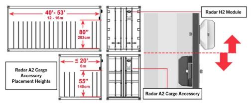
If your trailer is insulated (i.e., a reefer or heater) and you wish to avoid thermal losses caused from drilling through the door completely, we recommend limiting the depth of drilling and using Well Nuts, along with shorter bolts, to secure the device to the asset.
