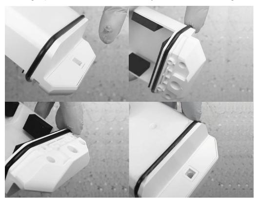
4. Completely insert the inner housing into the outer housing. Use the two screws that were provided with the device to secure the housing. **IMPORTANT:** Screw torque must be 3-3.5 in-lb. (0.35-0.4 N-m).
