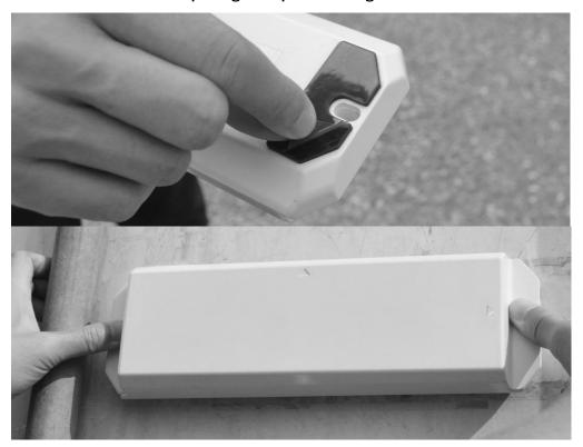
7. Insert your fastener of choice into the holes and use the appropriate tools to secure the module to the asset.
