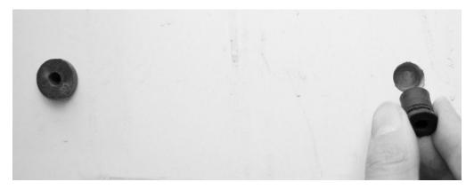
6. Remove the liner from the mounting pads, to reveal the adhesive. Place the module on the door, aligning the holes on the module with the holes you drilled into the door. **IMPORTANT:** This adhesive is intended only for temporary assistance during product installation. Do not attempt long term product usage without the use of fasteners.
