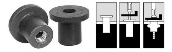
As you will need to supply two fasteners, you may determine which fastener is most suitable for your needs. Note: Your choice of fastener will influence the size of the tools required to create the mounting holes (i.e. drill bits) and install or remove the fasteners (i.e. wrenches/sockets/drivers). Likewise, the actual length of the fasteners will be determined by the thickness of your mounting surface and the fasteners selected. An example of this provided below.
