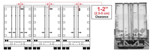
**IMPORTANT:** If you intend to pair your BlackBerry Radar H2 module with a BlackBerry Radar A2 Cargo Accessory, please ensure you do not install the BlackBerry Radar H2 module at a height that prevents the installation of the Radar A2 Cargo Accessory at the required placement heights in the illustration, below.
