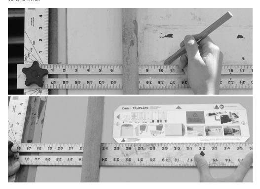
**Tip:** To avoid leaving a permanent mark on your trailer or container after the device installation is complete, we recommend using a pencil or non-permanent marker to create the guideline.
