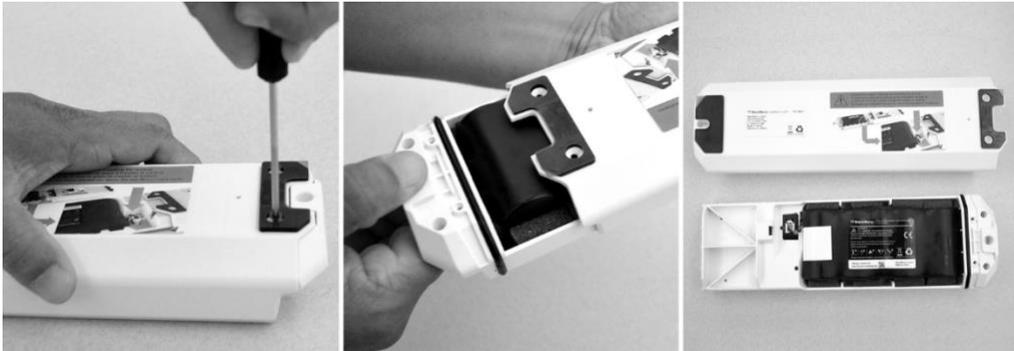
2. Ensure the battery cable is disconnected from the battery connector. Place the battery cable in the battery connector nest.
