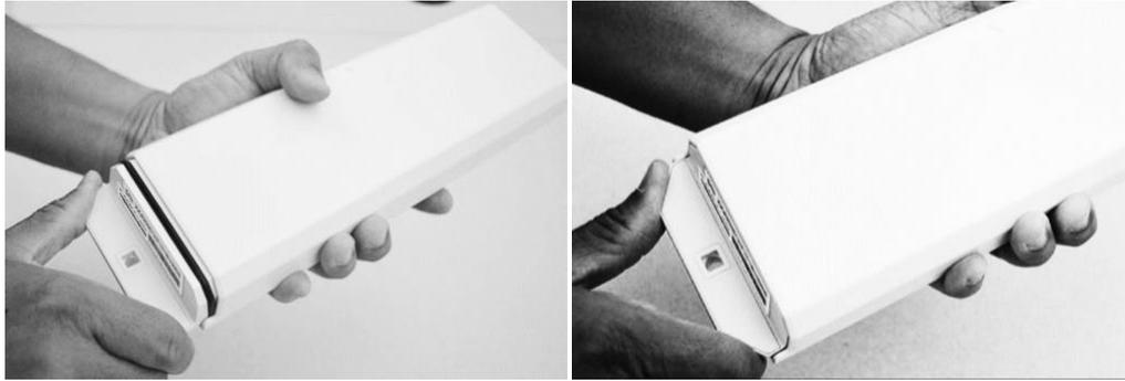
5. Locate the Fastener Bag and remove the two screws. Using a Phillips screwdriver, install the screws to secure the inner housing to the outer housing. **IMPORTANT:** Screw torque must be 3-3.5 in-lb. (0.35-0.4 N-m).
