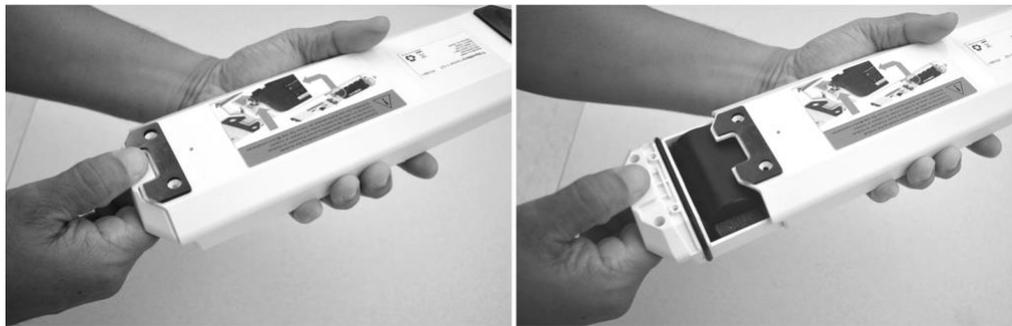
**Tip:** If you find it difficult to remove the inner housing from the outer housing, you may insert a tool, such as a screwdriver or long bolt, through the hole in the inner housing. Grasp the tool and the outer housing, then pull the two housings apart.
