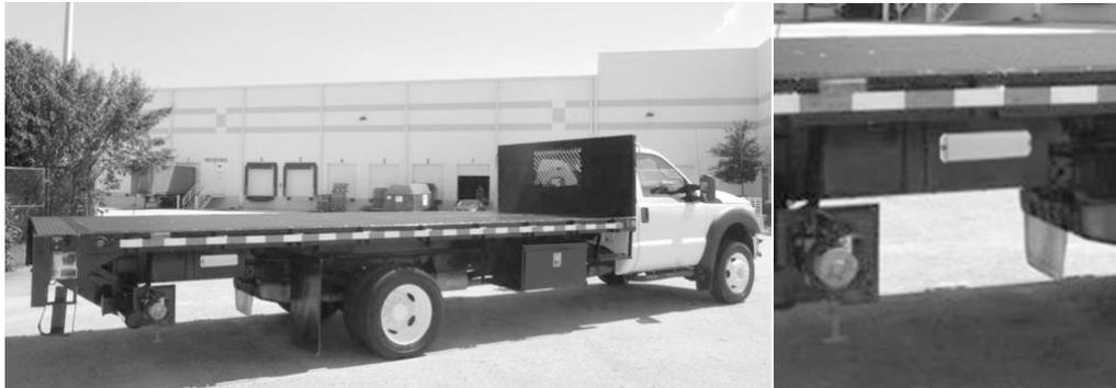
When looking for an installation location, if you are considering installation on a frame rail within an overhang, it is recommended to choose an installation location with a minimum clearance of 1/4" (6 mm) above and below the module. Maintaining this minimum clearance improves antenna performance. In some cases, as when installing on narrow width "C-channel" frame rails, it may be beneficial to mount the module on the opposite side of the frame rail to achieve the recommended clearance.
