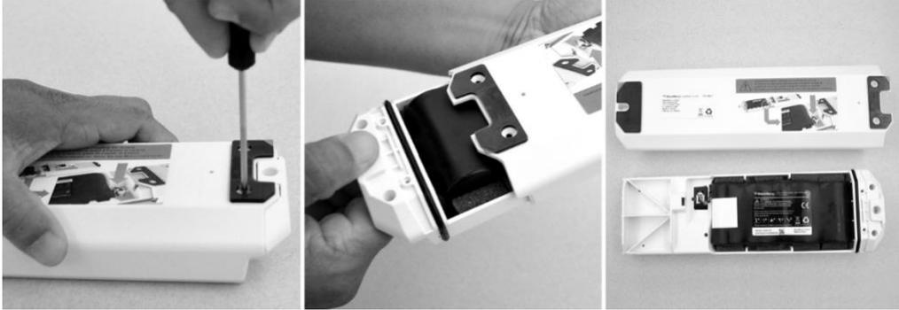
2. Disconnect the battery cable from the battery connector.
