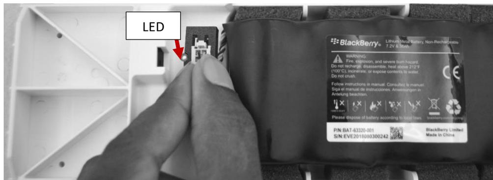
**IMPORTANT:** When connecting the battery cable to the battery connector, do not remove the Battery Connector Retaining Foam Retaining Tab or place the tab outside of
