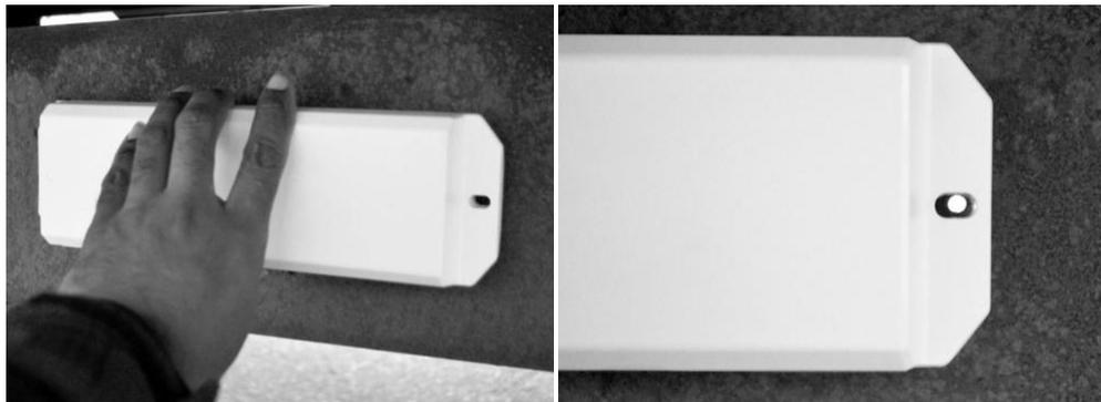
6. Insert your fastener of choice into the holes and use the appropriate tools to secure the module to the asset. Do not tighten fastener beyond 35 in-lb. (4 N-m).
