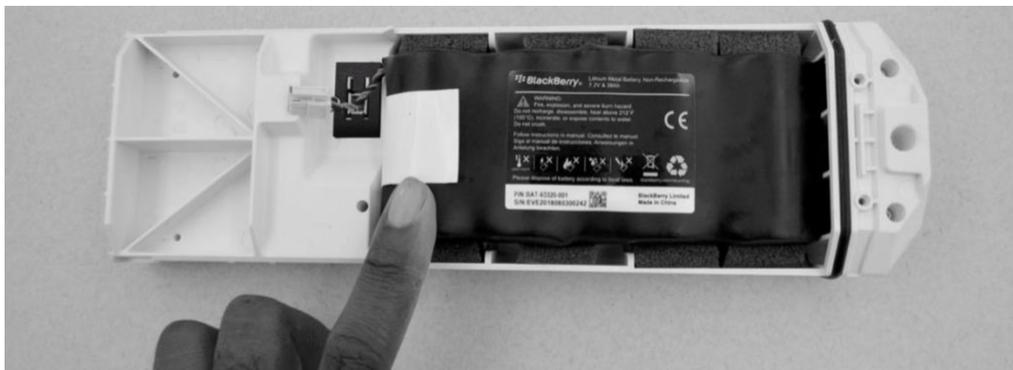
2. Connect the battery cable to the battery connector. The LED will blink to indicate the module is active. NOTE: It can take between 20-30 seconds for the blink sequence to begin. Please be patient. Once you see the LED blink, continue to the next step.
