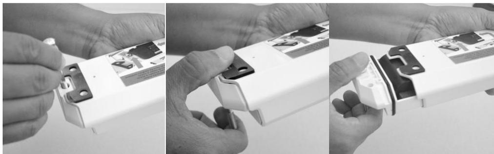
3. Remove the battery connector from the connector recess and connect the battery cable to the battery connector. The LED will blink to indicate the module is active. NOTE: It can take between 20-30 seconds for the blink sequence to begin. Please be patient. Once you see the LED blink, you may continue to the next step.
