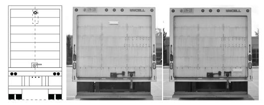
**IMPORTANT:** If you intend to pair your BlackBerry Radar H2 module with a BlackBerry Radar A2 Cargo Accessory, please ensure you do not install the BlackBerry Radar H2 module at a height that prevents the installation of the Radar A2 Cargo Accessory at the required placement heights in the illustration, below.
