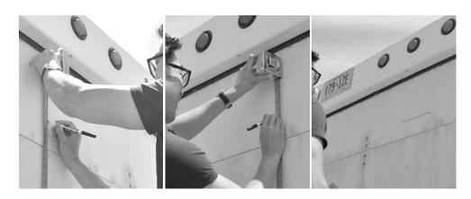
4. Remove the liner from the rear of the template and place the template in the desired installation location. The adhesive at the back of the template ensures that it stays on the door surface for accurate drilling of your holes.
