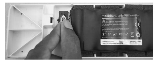
3. Remove the battery from the battery compartment by grasping the pull tab and lifting the battery out of the compartment.
