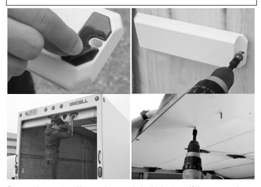
6. Remove the template. You now have two holes in the door. If there are any burrs around the holes, remove them at this time. Also, remove any dust or debris left over from the drilling or de-burring operations.
