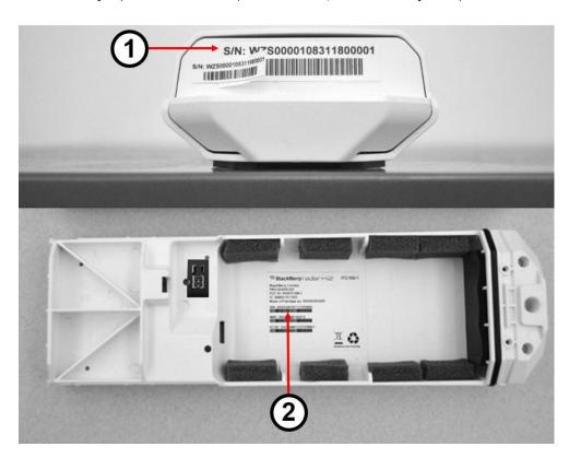
2. Once you are ready to install the module to the asset, remove the partially attached label from the front surface of the inner housing and place it on your worksheet, next to the asset identifier the module will be paired with.
