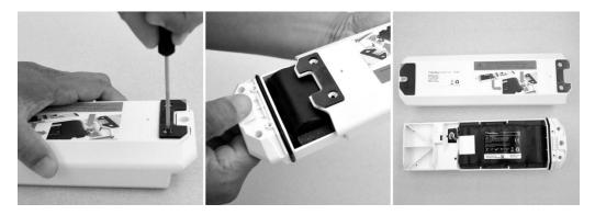
2. Disconnect the battery cable from the battery connector.
