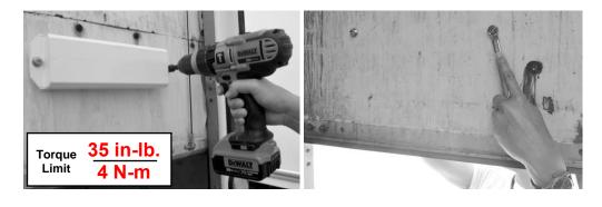
**IMPORTANT:** If you are using the lower door placement location, it is important to completely raise the door through its full range of travel, then lower the door completely, to initialize the door orientation sensor. Performing this operation allows the door to learn the difference between a door open and door close event.
