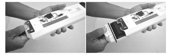
**Tip:** If you find it difficult to remove the inner housing from the outer housing, you may insert a tool, such as a screwdriver or long bolt, through the hole in the inner housing. Grasp the tool and the outer housing, then pull the two housings apart.
