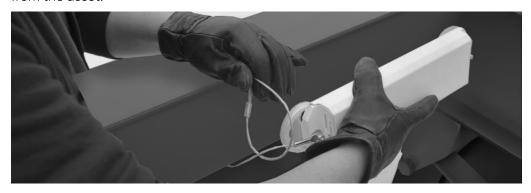
2. Loosen the large loop on the tether, then draw the module through the loop.
