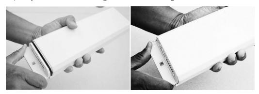
5. Locate the Fastener Bag and remove the two screws. Using a Phillips screwdriver, install the screws to secure the inner housing to the outer housing. **IMPORTANT:** Screw torque must be 3-3.5 in-lb. (0.35-0.4 N-m).
