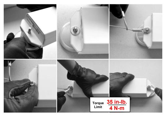
**IMPORTANT:** Do not over-tighten the fasteners. Do not tighten beyond 35 in-lb. (4 N-m). Over-tightening can lead to mis-alignment of the magnet, which may reduce the holding power of the magnet.
