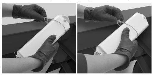
3. Using the magnets, attach the module to the asset.
