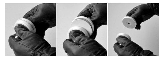
**Tip:** To avoid unintended attraction of the two magnets to each other, and other magnetic materials in the vicinity, we recommend temporarily returning the second magnet to the packaging insert, while you install the first magnet to the device.
