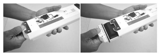
**Tip:** If you find it difficult to remove the inner housing from the outer housing, you may insert a tool, such as a screwdriver or long bolt, through the hole in the inner housing. Grasp the tool and the outer housing, then pull the two housings apart.
