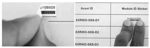
**Tip:** For modules that have previously been transferred to new assets, the temporary S/N label may no longer be in place. If this is the case, you will need to write the module identifier (S/N) for each module on the installation worksheet.
