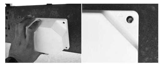
6. Insert your fastener of choice into the holes and use the appropriate tools to secure the module to the asset.
