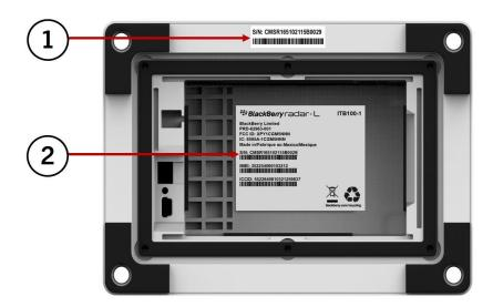
2. Once you are ready to install the module to the asset, remove the partially attached label from the outer surface of the rear housing and place it on your worksheet, next to the asset identifier the module will be paired with.
