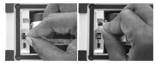
3. Remove the battery from the battery compartment by grasping the pull tab and lifting the battery out of the compartment.
