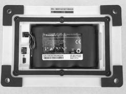
3. Remove the battery connector from the connector recess and connect the battery cable to the battery connector. The LED will flash to indicate the module is active.
