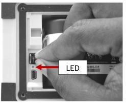
4. Re-install the battery cover using the six screws that were supplied with the module. **IMPORTANT:** Screw torque must be 4.4 in-lb. (0.5 N-m).
