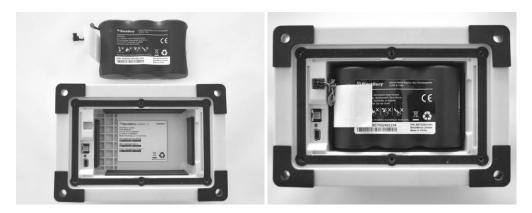
2. Connect the battery cable to the battery connector. The LED will flash to indicate the module is active.
