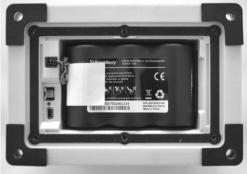
2. Ensure the battery cable is disconnected from the battery connector. Place the battery cable in the battery connector nest.
