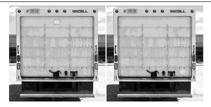
3. Once you have identified the desired mounting location for your asset, mark the height where the device will be installed on the door of the trailer/container.
