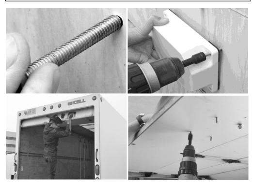
6. Remove the template. You now have four holes in the door. If there are any burrs around the holes, remove them at this time. Also, remove any dust or debris left over from the drilling or de-burring operations.
