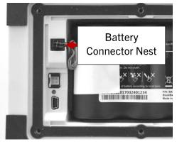
3. Place the battery cover onto the module and install all six screws. Module is now ready to be placed in the UN certified Dangerous Goods packaging.
