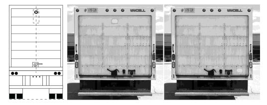
If your trailer is insulated (i.e., a reefer or heater) and you wish to avoid thermal losses caused from drilling through the door completely, we recommend limiting the depth of drilling and using Well Nuts, along with shorter bolts, to secure the device to the asset.
