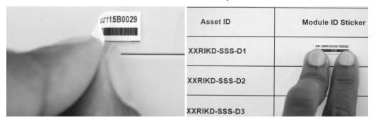
**Tip:** For modules that have previously been transferred to new assets, the temporary S/N label may no longer be in place. If this is the case, you will need to write the module identifier (S/N) for each module on the installation worksheet.
