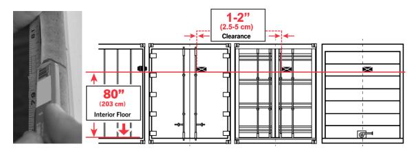
\* **Note:** Location of the module is critical to its performance. Please ensure the bottom of the device is installed 80" (203cm) above the interior floor.
