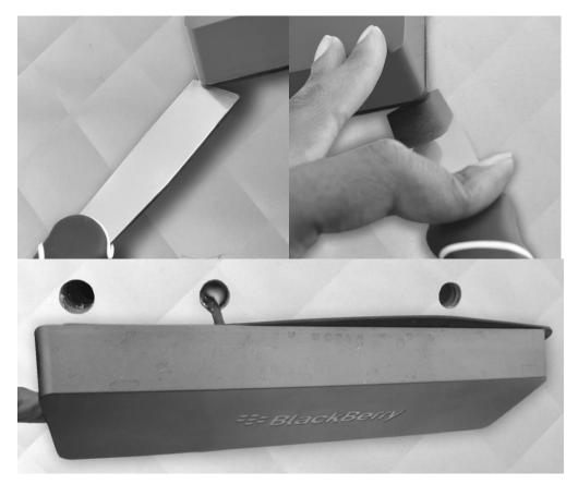
C. From inside the trailer, use the screwdriver to push on the sealant to force the sealant through the hole and out the rear of the trailer. When enough of the sealant plug is outside the hole, from outside the trailer, pull the sealant from the hole and guide the cable through the hole to complete removal of the module from the trailer.
