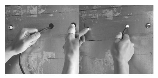
**Tip:** If you choose to use Technique 1 for module removal, you may wish to place a rag, or block of wood between your hand and the screw boss for added comfort while pushing on the module.
