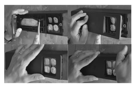
**IMPORTANT:** After the device has been completely installed, be sure to completely close all doors of the trailer/container. Closing the doors, will begin the process of baselining the cargo load state. For optimal results, be sure to keep the doors closed for 20 minutes to allow adequate time for the process.
