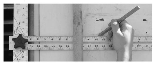
**Technique 2:** Alternatively, you may use tape to extend the mark from the edge of the door, to the exterior surface of the container. This can be helpful if you do not have enough clearance to fit the T-square between the door and the locking bar.
