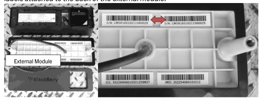
2. Locate your installation worksheet. Remove the partially attached label from the rear of the external module and place it on your worksheet, next to the asset identifier the device will be paired with.
