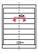
5. Remove the adhesive liner from the drill template. The adhesive at the back of the template ensures that it stays on the door surface for accurate drilling of your holes. Align the perforated edge of the template along your mark. Allow approximately 1-2" (2.5-5cm) of clearance between the left side of the template and the edge of the door bar. Ensure the template is level.
