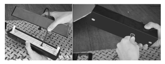
3. Remove the screws from the external module.
