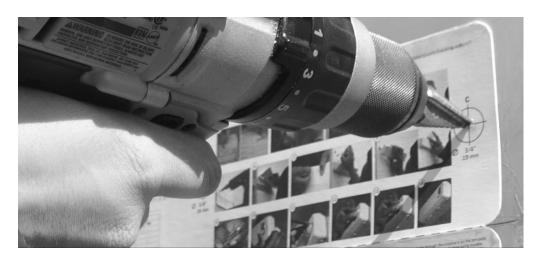
**Note:** For shortest drilling time, and burr-free holes, we recommend using a step drill bit. Step drill bits also offer improved drilling speed through the harder steel used on intermodal containers. To further shorten drilling time and prolong the life of your drill bit, you may wish to apply Cutting Tool Lubricant to your drill bit prior to drilling.
