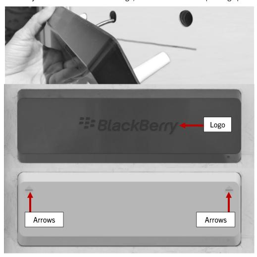
11. Apply firm pressure to the external module for 30-45 seconds to ensure it adheres to the wall. The adhesive will hold the external module in place while you complete the installation.
