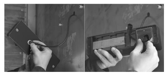
15. Place the internal module onto the screw bosses. Use the screws to fasten the external module to the internal module. Do not overtighten the fasteners. Do not exceed 48 in-lb. or 5 N-m.
