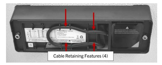
**Tip:** When placing the cable connectors inside the cable connector recess, take care to avoid crossing the cable over itself. Doing so can make it more difficult to secure the cable and attach the lid.
