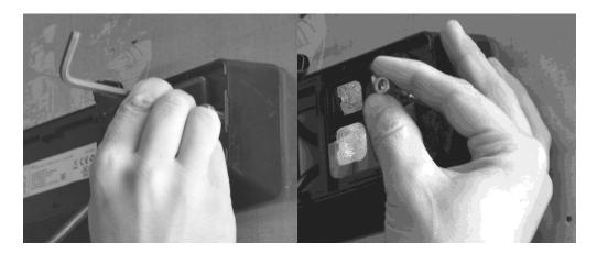
5. Remove the internal module from the door. Guide the internal module along the cable and the connector through the hole on the internal module.
