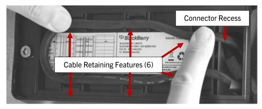
**Note:** When installed on reefer trailers, not all of the cable retaining features will be occupied as more cable will be consumed inside the thicker door. The following image shows the cable management after installation on a reefer door.
