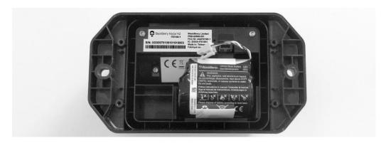
2. Connect the battery cable to the battery connector. The LED will blink to indicate the module is active. **NOTE:** It can take up to 5 seconds for the blink sequence to begin. Please be patient. Once you see the LED blink, continue to the next step.
