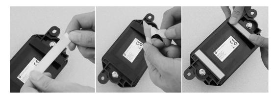
9. Remove the clear liner. Align the holes on the 20° bracket to the areas you marked on the wall and place the module on the prepared mounting surface. Apply firm pressure (15 psi) to the module for 30-45 seconds to ensure the adhesive bonds to the surface.
