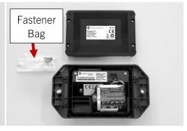
**Tip:** If you find it difficult to remove the inner housing from the outer housing, you may insert a tool--such as a screwdriver--near the arrows embossed into the door and lift to separate the door from the housing.
