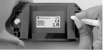
3. Remove the white extended liner from the back of the tape. Apply to the battery door. Using firm pressure (minimum of 15 psi) to ensure adhesive bonds to battery door.
