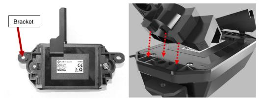
7. Secure the bracket and visor to the R2 module. Do not tighten fastener beyond 35 in-lb. (4 N-m).
