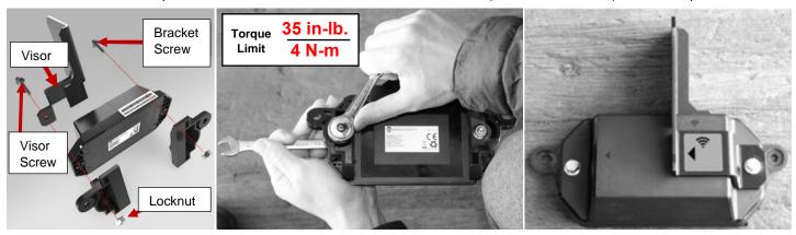
8. Re-install R2 module and visor assembly to the asset, using the tools and fasteners of your choice.
