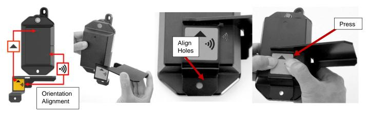
6. Re-install the bracket that was removed in Step 3 to the rear of the Radar R2 module, ensuring the holes on the R2 20° Tilt Bracket are aligned with the holes on the R2 module and visor and the bracket's guide tabs are seated within the rear openings of the module.
