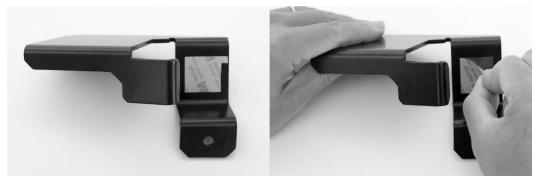
5. Align the orientation of the arrow and signal icon on the visor with the arrow and signal icon on the Radar R2 module. Place the visor onto the device, ensuring the hole on the visor is aligned with the hole on the device. Press the center of the label to activate the adhesive.
